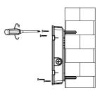
8. Push the expansion rubber plug into the mounting hole on the wall
