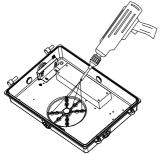
5. Drill through the mounting hole with an electric drill.
