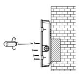
8. Lock the bottom shell on the mounting seat with screws.
