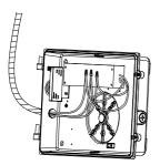
9. Connect the top terminal to the wire tube through the side hole to the L, N and G wires on the power supply.
