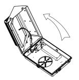
3. Open the fixture, disconnect the connection terminals, and remove the upper cover of the fixture.
