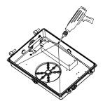
4. Drill through the mounting hole with an electric drill.
